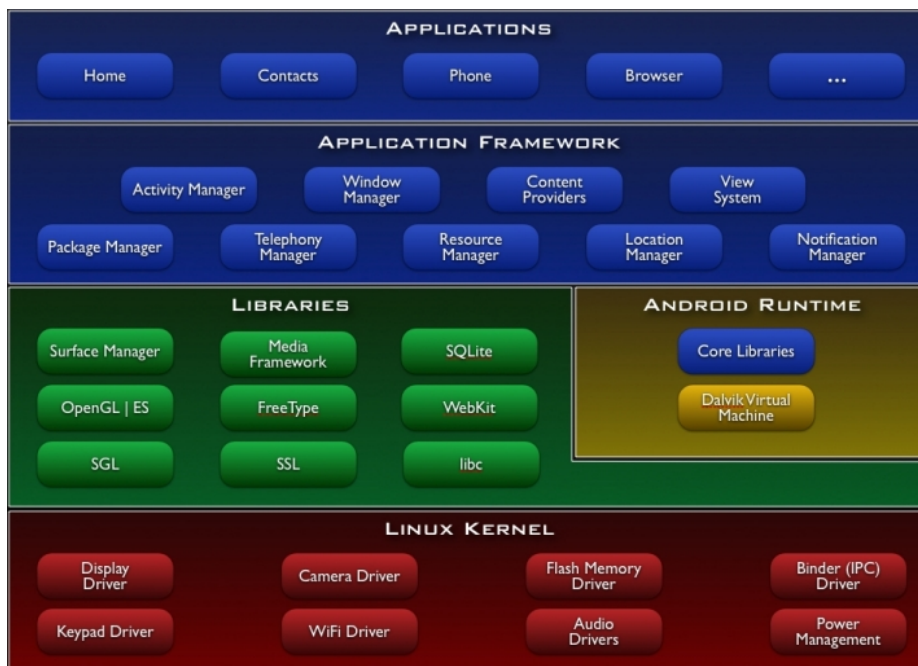
Fig. 1. System architecture of Android [6]
